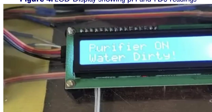
Figure 5. LCD Display showing purifier activation status
