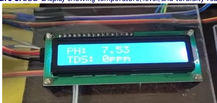
Figure 4. LCD Display showing pH and TDS readings
