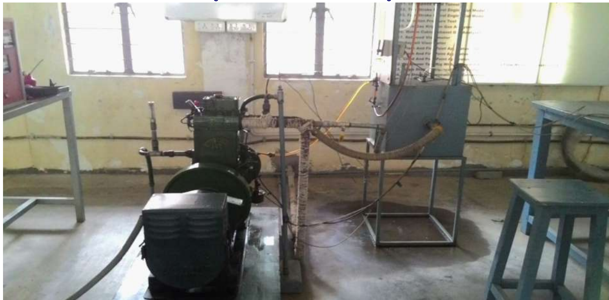
Fig. No.: 9.2. 4- Stroke Diesel Engine Test Rig
