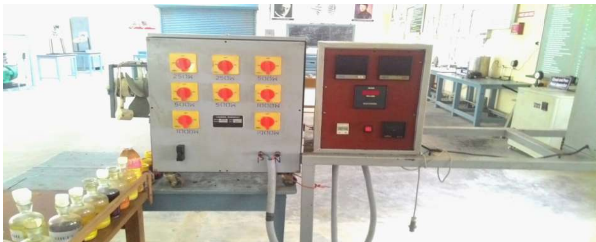
Fig. No.: 9.3. Electrical Circuits for Engine Test Rig
